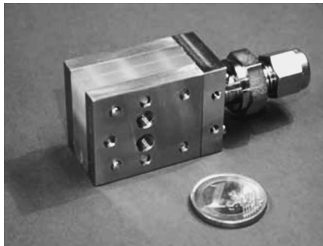
Fig. 7. Caterpillar mixer with straight outlet (source: IMM).
